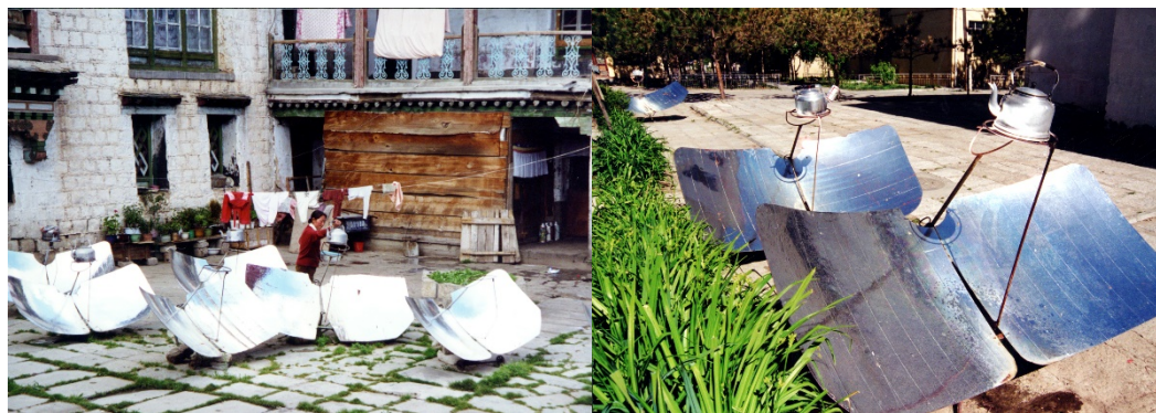
Fig. 1 Application of solar cooker in Tibet
