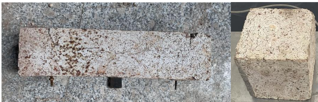
Fig. 4 Apparent characteristics after being subjected to fire for 60 min
