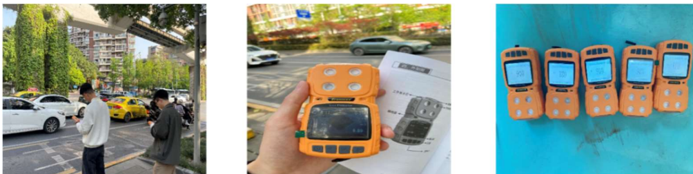
Figure 2. Trial and Calibration of Handheld Gas Detectors
