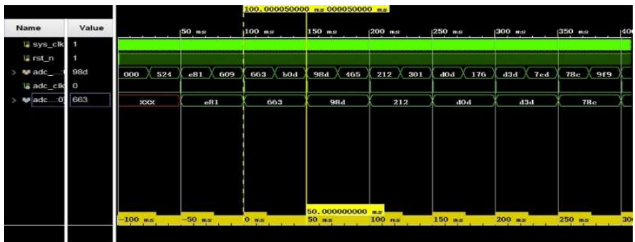
Figure 4. Simulation diagram of AD9226 data acquisition
