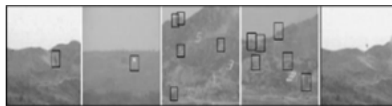
Figure 8. Results of double CCD detection of blast points
