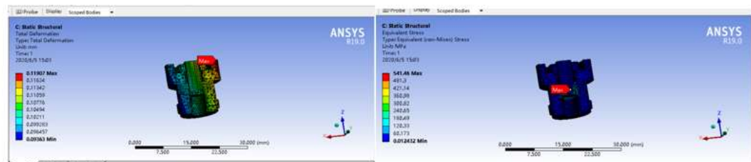
Figure 16. Stress-strain diagram of sensor at thickness of 7mm
