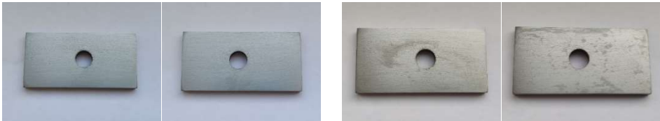
Figure 10. Appearance of cast iron before and after corrosion test
