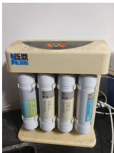
Figure 4. Reverse osmosis deionization water purifier
