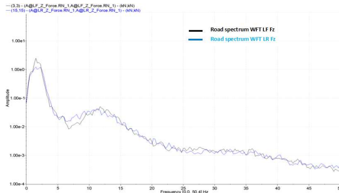
Figure 7. LF and LR WFT Fz channel data frequency domain diagram
