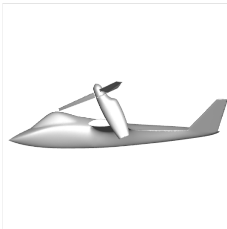
Figure 15. Tilt-rotor aircraft with an Engine Nacelle Deflection of 60^\circ
