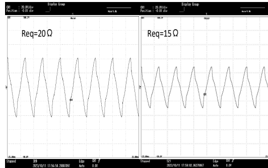
Figure 18. the relationship between the output voltage and the load in the constant current mode.
