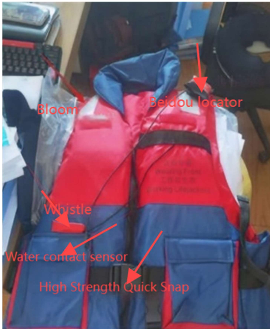
Fig. 2 Low-power life-saving dedicated two-way BeiDou Terminal
