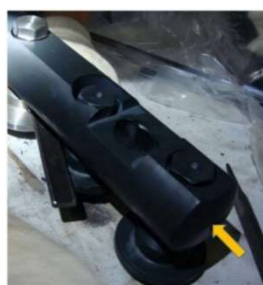
Figure 10. Valve Beam End Face and Steam Impact Zone
