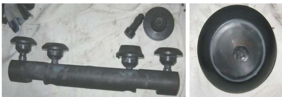
Figure 2. V-Valve Stem Fracture and II-Valve Disc Scar
