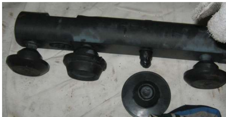
Figure 6. Fracture photo of V-Valve Stem
