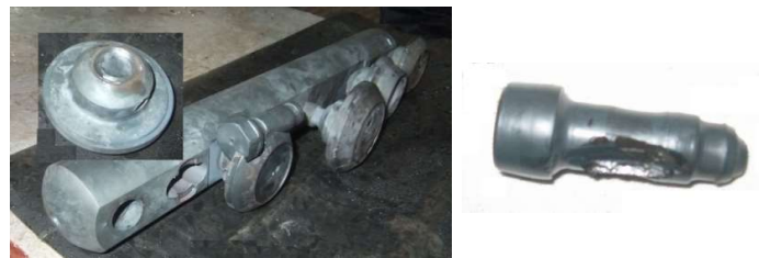
Figure 7. Fracture Diagram of IV-Valve Stem
