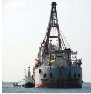
Figure 3. “Lan Jiang”Pipe Laying Crane
