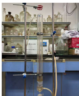
Fig. 1. Measuring device for foaming force and foam stability of foaming agent
