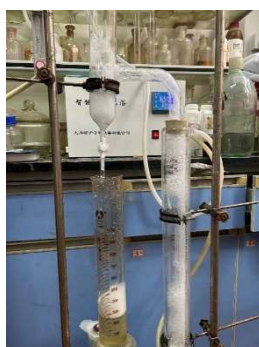
Fig. 2 Liquid carrying capacity measuring device for foaming agent
