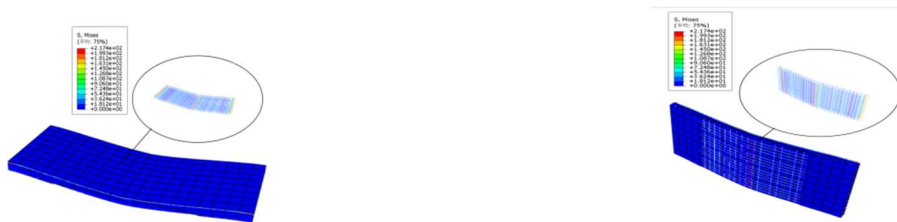
(a) Cloud diagram of principal stress distribution on the traveling surface (b) Cloud map of principal stress distribution on the spalled surface
