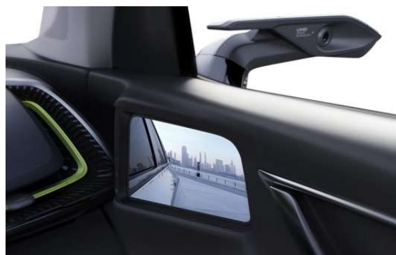
Fig. 1 The CMS equipped on a certain model of automobile.
