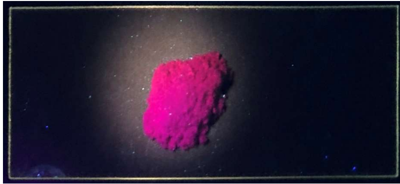
Fig. 4 Luminescence photograph of \text{Na}_{0.99}\text{Li}_3\text{SiO}_4: 1\% \text{Mn}^{2+} sample under UV irradiation at 365 nm
