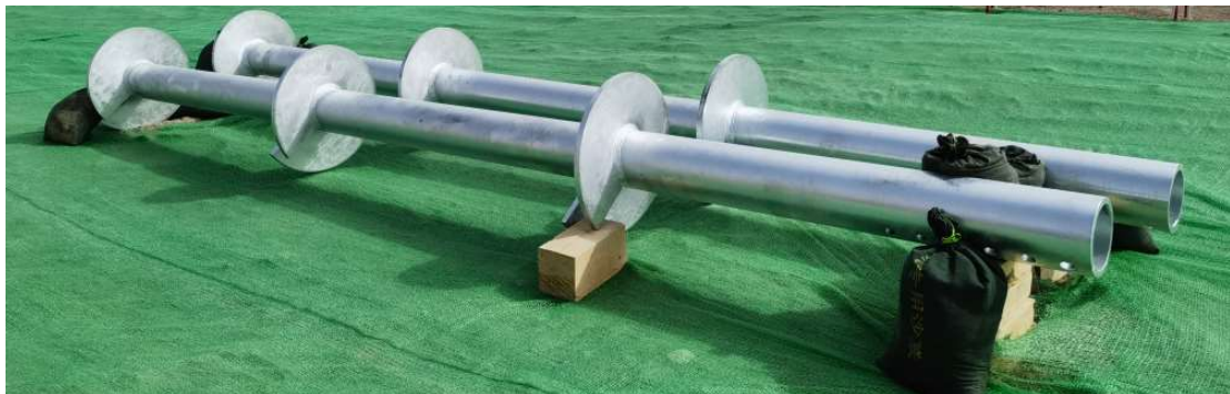
Figure 2. Composition of Single Helical Anchor
