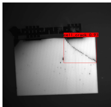
(b) Battery crack detection results after model optimization
