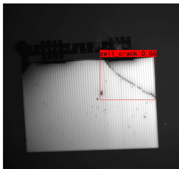
(a) Battery crack detection results before model optimization
