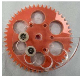
Figure 3. Actual image of the cam (the transparent part is the cam, the pink part is the gear)
