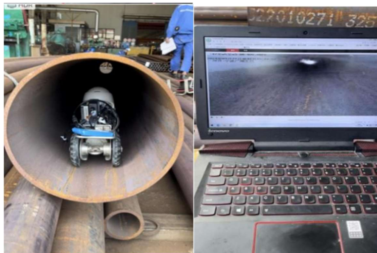
Figure 5. Testing for the Pipe-line Inspection
