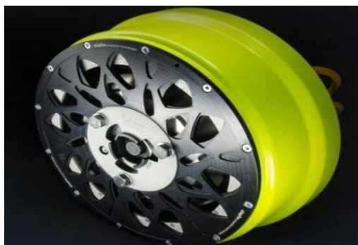
Fig. 4 Zhejiang Asia-Pacific In-Wheel Motor M700.
