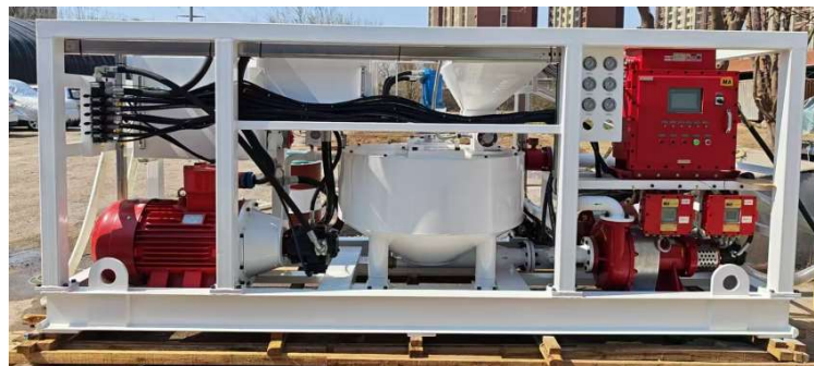
Fig. 5 Physical diagram of the sand-mixing sled prototype
