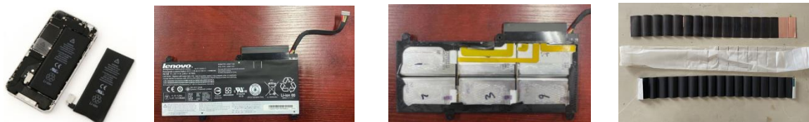
Fig. 11 Disassemble the lithium battery
