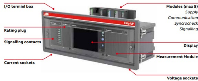
Figure 2. Ekip UP Digital upgrade unit
