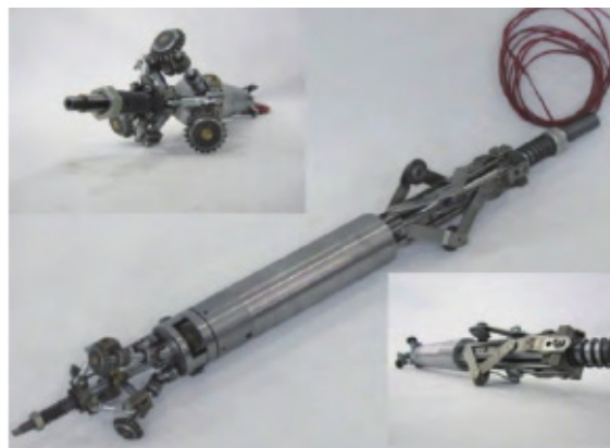
Figure 9. Active spiral pipeline robot
