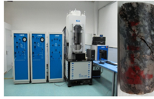
Figure 1. Rock Mechanics Experiment Equipment and Experimental Rock Samples
