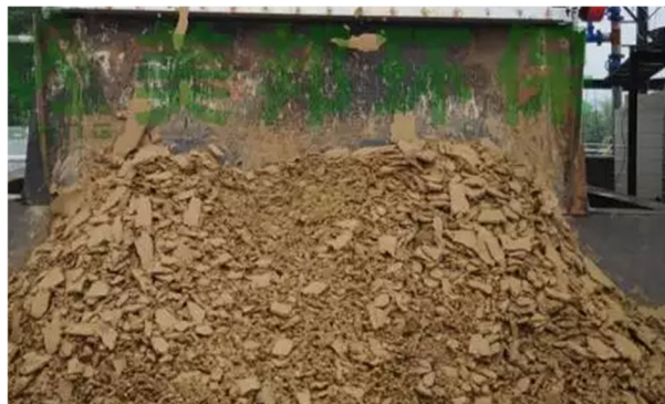
Figure 4. Effect diagram of shield muck after pressure filtration treatment
