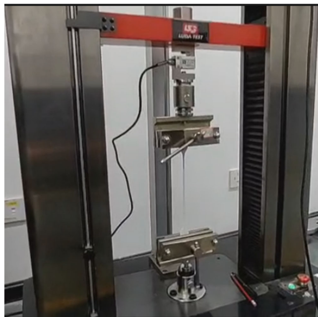
Figure 5. Rubber specimen tensile test (universal testing machine)
