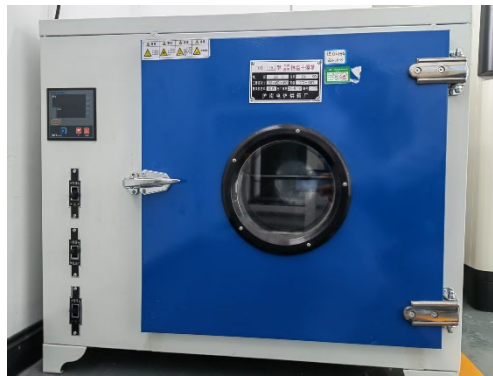
Figure 3. Constant temperature drying oven
