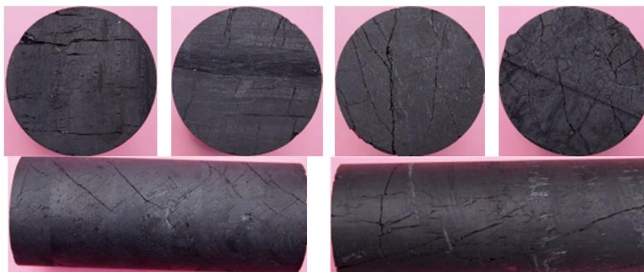
Figure 3-2. A cylindrical specimen with a diameter of 50 × 70mm from the Ba Mine coal mine
